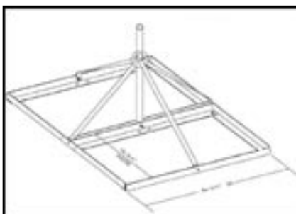
Figure 9. Rohn/Radian FRM238 non-penetrating mount.
